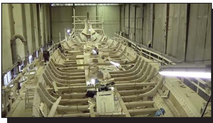
6 standing knees are used in the foreship and reach over the gunwale and become bollards for mooring. 10 boatbuilders worked over 20 months to get to this stage shown below
