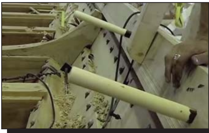
Standing knees must be shaped to the hull, stringer and the cross braces. The stringer is attached to the planking with wood nails
