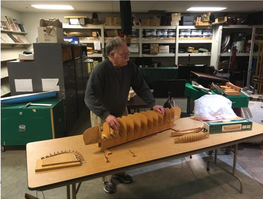
Mike explained that he always wanted to build a full size canoe from scratch and did the model version as a warm up. Based on plans from Ted Moores, Bear Mountain Boats, Mike adjusted scale on a copy machine for the various sized forms in the photo. The canoe was actually completed about a year ago. Here is the finished boat:
