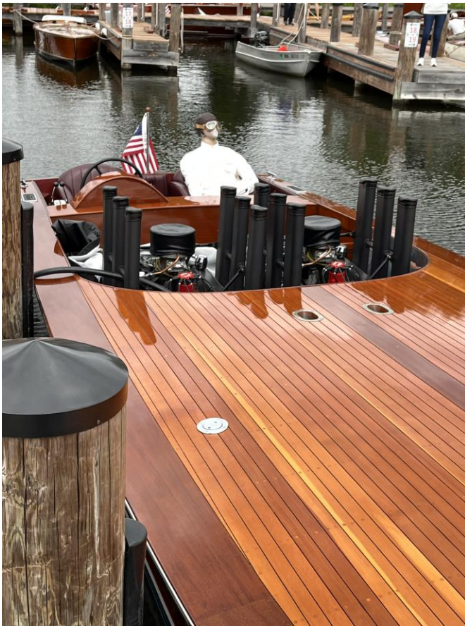
Miss America IX, the first boat to exceed 100 mph, in 1931. It is a single step hydroplane, done with twin Packard V-12 engines, now sporting twin big block Chevrolet engines. Note the skipper was well protected!
