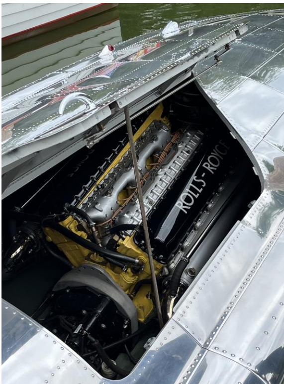
The Hornet II is a 1930 Gar Wood with a Rolls Royce V-12 engine, and it sounded glorious with the unmuffled side pipes!
