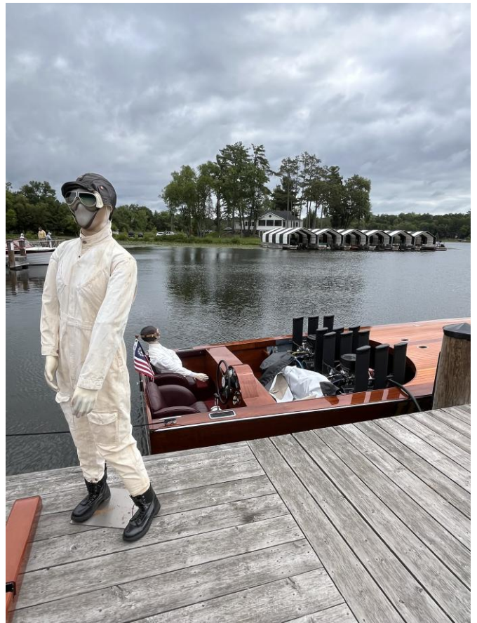
Miss America IX, the first boat to exceed 100 mph, in 1931. It is a single step hydroplane, done with twin Packard V-12 engines, now sporting twin big block Chevrolet engines. Note the skipper was well protected!
